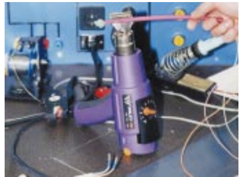
Shrinking a PVC heat-shrink tube with reflector.
